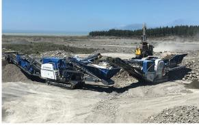
Figure 34 - Mobile screening plant
