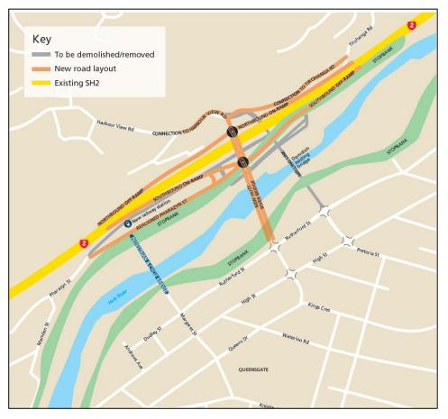
Figure 19 - New diamond interchange at Melling
